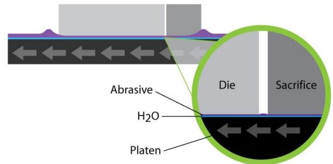
*Figure 8: This illustration shows how the bulging and thus overpolish is reduced when using a thinner backed abrasive.*
